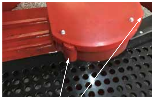
Easy changable screen with PU bumpers.
