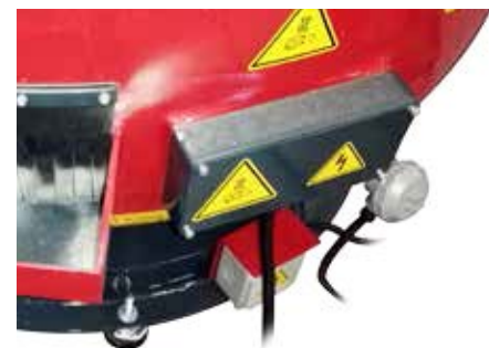
Resistance - electrical box with thermocouple.
